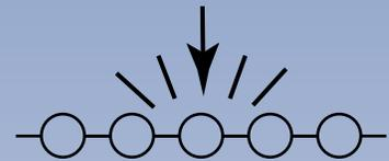
Cross section of Aquasol collector showing the closely spaced tubes and interconnecting webs, which expose more surface area to the sun, resulting in higher performance. The interconnecting webs also relieve the thermal stress of expansion and contraction, assuring years of trouble-free operation
